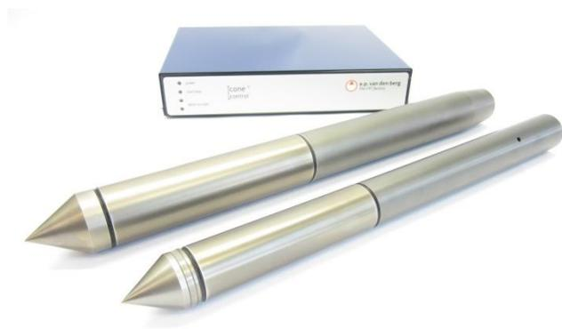
required for the wave to reach the seismic sensors is recorded. The time difference between two consecutive seismic tests performed is a measure of the elastic properties of the soil. An even faster and more accurate way is to use two seismic modules which are mounted at a fixed distance of exactly 1 meter.
