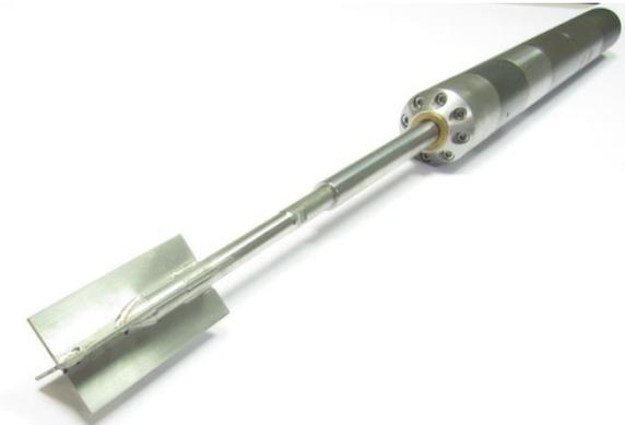
Fig. 10. Icone vane (without protection tube).
