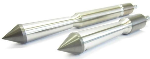
The electrical cone is pushed into the soil with a constant rate and is therefore a more straightforward and faster way of soil investigation in comparison with the mechanical cone. Furthermore the real time processing and visualizing of the data obtained, facilitates a better control over the CPT-process.
