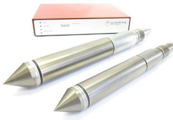
connectors and the data logger. The calibration settings are essential for a good data processing and must be read from a USB-memory stick into the data processing computer system. Accidentally changing of calibration settings and getting rid of the USB-stick may lead to errors. Finally the electrical cone is more expensive compared to the mechanical cone, so financial losses are higher in case a cone breaks off.
