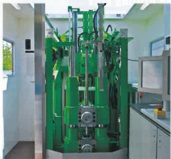
Modern systems work with the aid of hydraulic cylinders pushing the specially shaped CPT cone into the ground at a constant (2cm per second) speed. The cone information is fed back to a computer, the data recorded and interpreted accordingly. Depending on what is required, different cones are used or a single cone is extended by adding modules to measure the various parameters.
